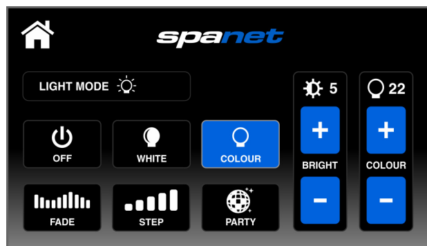
User Colour Mode Select from 30 possible colours (RH slider) Light brightness adjustment (LH slider)
