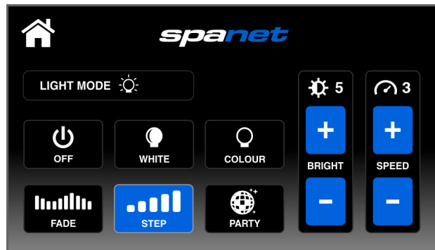
Step Effect Step transition through all possible colours Light effect transition speed (RH slider) Light brightness adjustment (LH slider)
